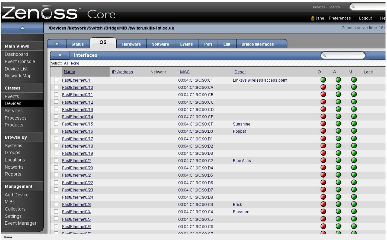
Figure 46: Standard OS tab for switch device with MIB-2 interfaces in Zenoss 2
