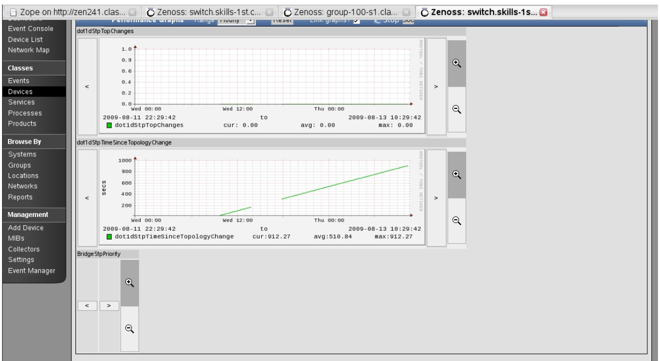
Figure 105: The empty graph at the bottom suggests that a template is bound but no data has been collected
