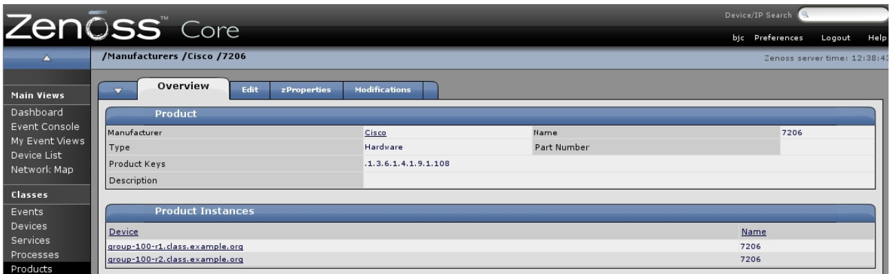
Figure 8: Product entry for Cisco 7206 router showing SNMP OID association
